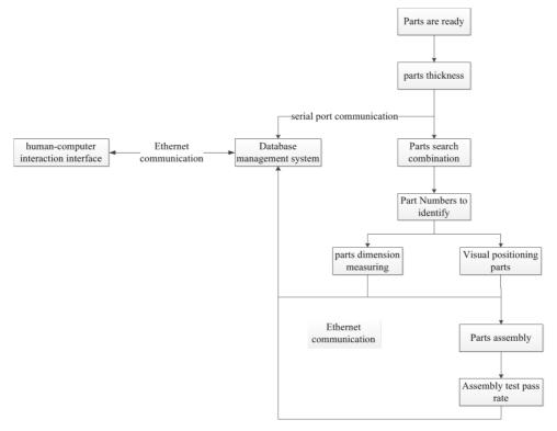
Fig. 1. Overall block diagram of the system
